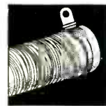
Lack of accuracy in pitch or tension will cause shorted turns or
