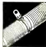
Control of these factors is perfect. Two wire sizes are often wound on one tube.
